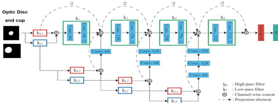
Figure 3: Deep Wavelet Scattering Network
