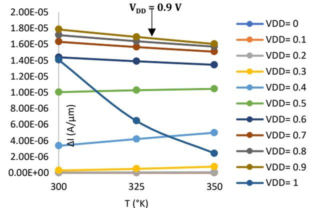
FIGURE 6. ΔI-T FinFET characteristics (Wg =10nm, Lg=20nm).
