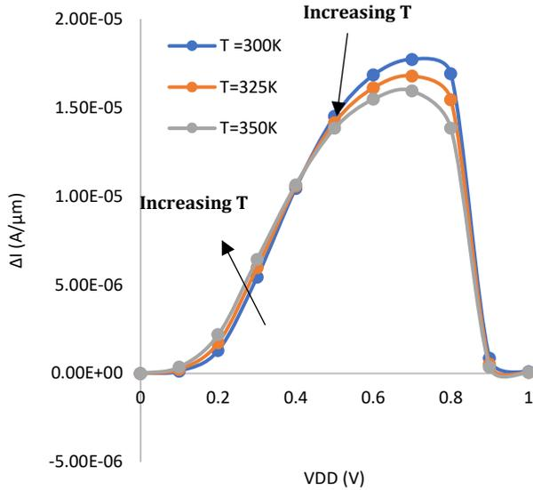
FIGURE 8. FinFET characteristics ( $W_g=10\text{nm}$ ,  $L_g=10\text{nm}$ )  $\Delta I-V_{DD}$ .
