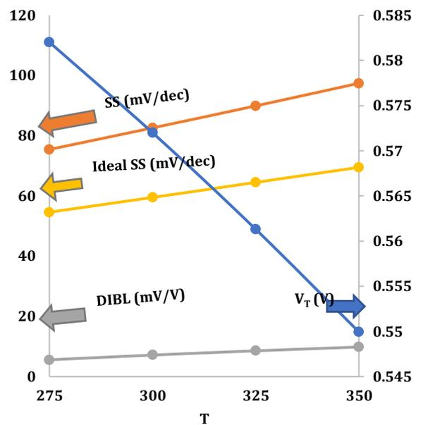
FIGURE 14.  $V_T$ , SS and DIBL at  $W_g=10\text{nm}$ ,  $L_g = 30 \text{ nm}$ .)
