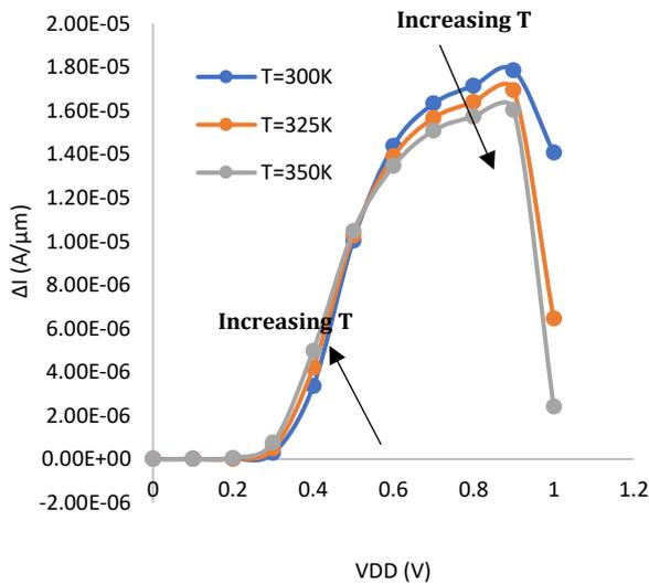
FIGURE 9. FinFET characteristics ( $W_g=10\text{nm}$ ,  $L_g=20\text{nm}$ )  $\Delta I-V_{DD}$ .
