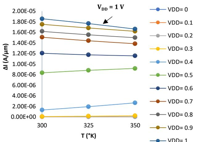
FIGURE 7. ΔI-T FinFET characteristics (Wg =10nm, Lg=30nm).
