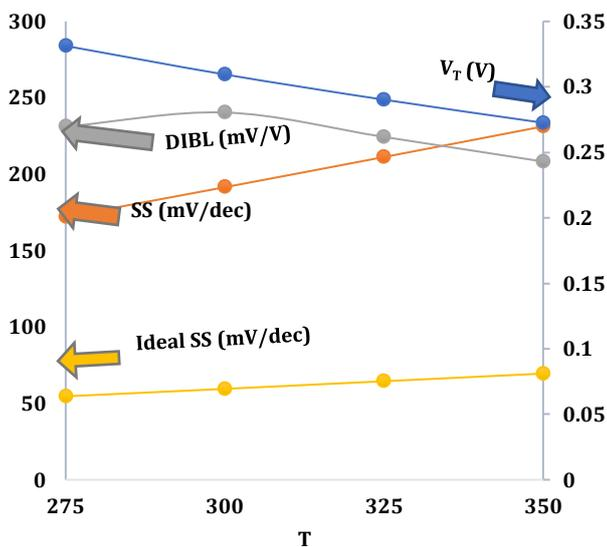
FIGURE 12.  $V_T$ , SS and DIBL at  $W_g=10\text{nm}$ ,  $L_g = 10 \text{ nm}$ .)
