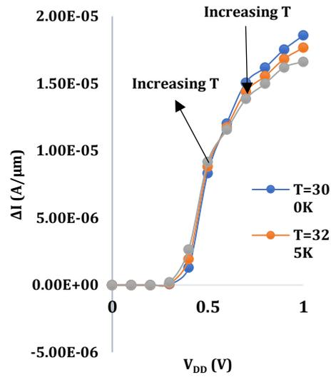
FIGURE 10. FinFET characteristics ( $W_g=10\text{nm}$ ,  $L_g=30\text{nm}$ )  $\Delta I-V_{DD}$ .
