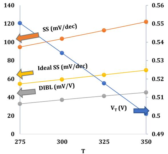
FIGURE 13.  $V_T$ , SS and DIBL at  $W_g=10\text{nm}$ ,  $L_g = 20 \text{ nm}$ .)
