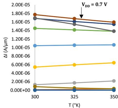
FIGURE 5. ΔI-T characteristics of FinFET (Wg=10nm, Lg = 10nm).
