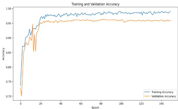
FIGURE 13. Accuracy curves of the ResNet50 in the triple classification.
