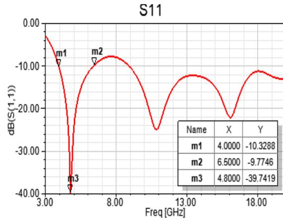
FIGURE 2. The performance of return loss at a frequency of 4.80 GHz
