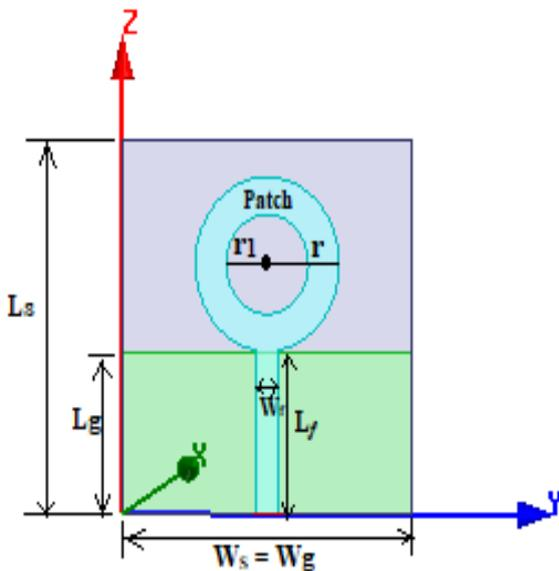
FIGURE 1. Structure of the proposed antenna
