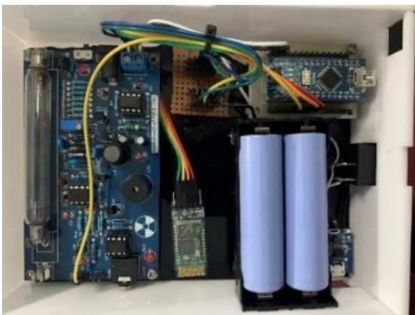
FIGURE 4 The entire measurement module using Geiger Muller sensor for X-ray radiation measurement.
