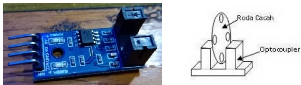
FIGURE 6. Optocoupler Sensor and Wheel Encoder
