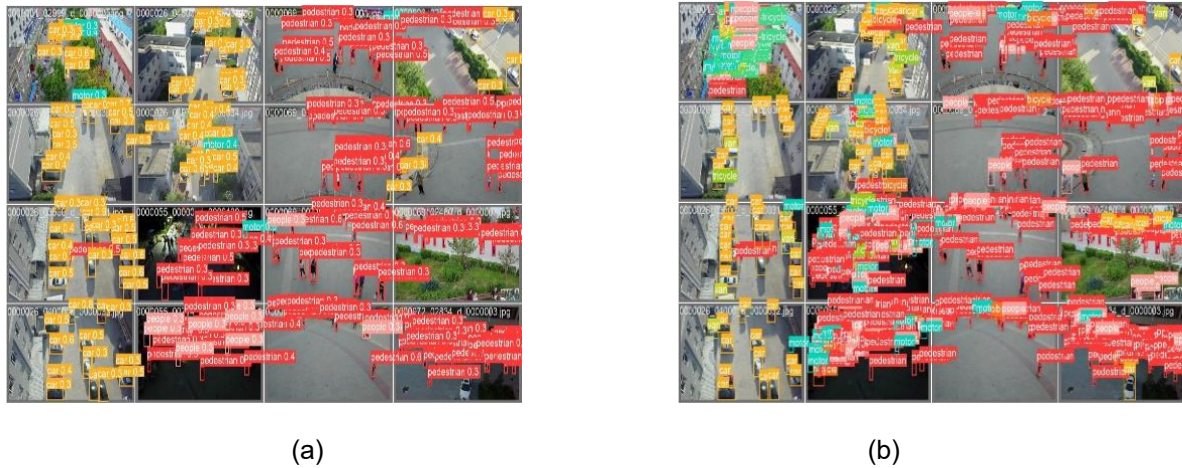
Fig. 11. Demonstrates YOLOv8-SR effectiveness in the recognition of the targets in (a) Validation Labels, and (b) Validation Predictions.
