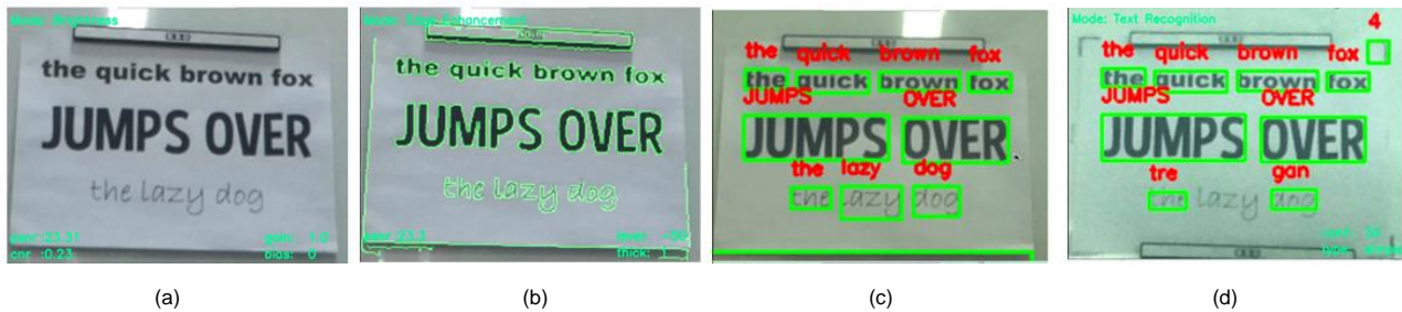
FIGURE 2. Image processing results from camera view: (a) Brightness mode, (b) Edge enhancement using thresholding of 10 and level of -50, (c) Text detection in light condition, and (d) Text detection in dark condition.
