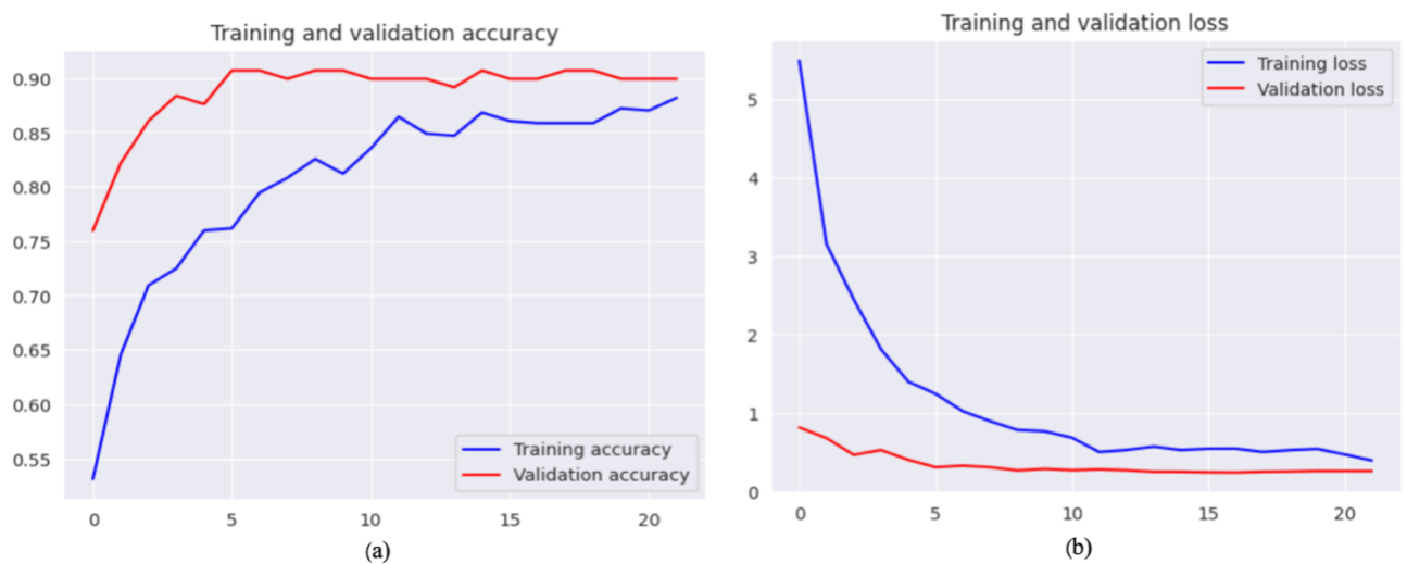
Fig. 7. Epoch results using MobileNetV3 architecture: (a) Accuracy vs. epoch; (b) Loss vs. epoch
